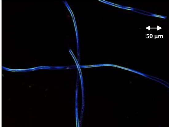
Acrylic fibers mounted in 1.527 HD liquid
