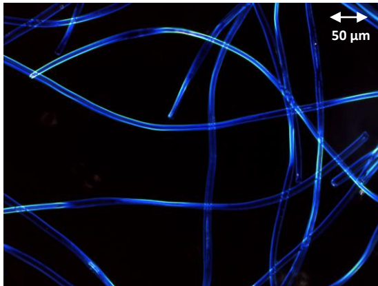
Modacrylic fibers mounted in 1.550 HD liquid
