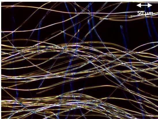
Silk fibers mounted in 1.550 HD liquid
